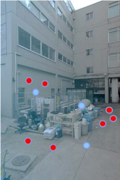
Fig. 5: 3D data view from the scanner image. Both the scanned point cloud and the SFM/MVS reconstructed meshes can be selected from the same pixel section, which permits correspondences to be easily made via mouse picking.
