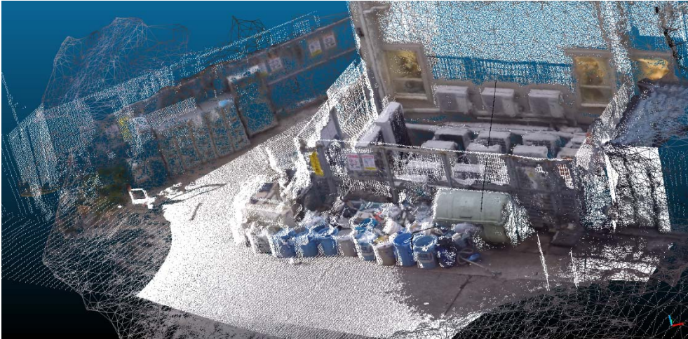
Fig. 6: Registration result. The white dots show the point cloud produced by the scanner and the colored dots are the SFM/MVS reconstruction.
