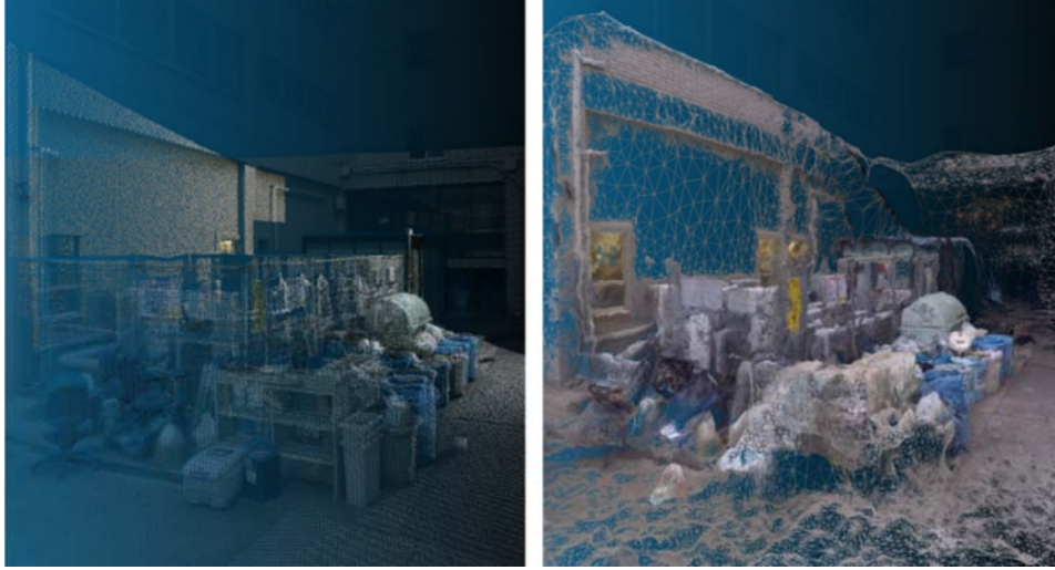
Fig. 4: Point cloud data view (left) and reconstructed meshes view produced by a SFM and MVS process from an identical viewpoint obtained via the scanner camera. Corresponding points can be found at the same pixel position on the image.
