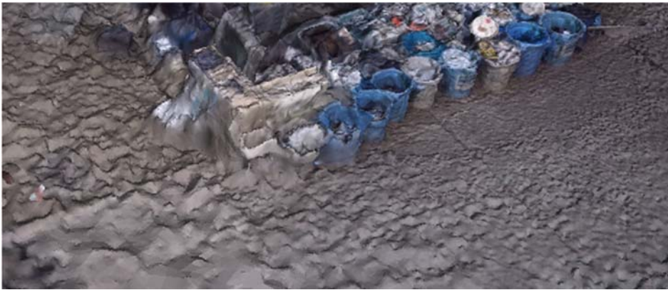
Fig. 7: Artifacts in the reconstructed SFM and MVS meshes. Reducing the number of image features may cause more unevenly shaped artifacts on originally smooth surfaces.
