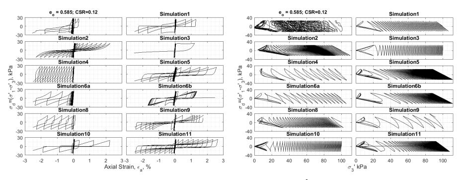
cyclic stress-controlled test on Ottawa F65 sand for  $\rho_d$ =1,666 kg/m³, (e= 0.585, Dr~71.5%), p'<sub>0</sub>=100 kPa, CSR=0.12.
