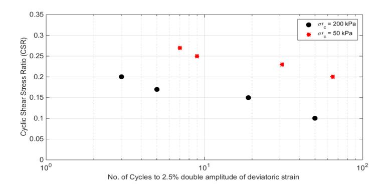
Cyclic undrained traixial tests conducted on Ottawa F-65 sand with an average initial density of 1658 kg/m³ (Vasko, 2015).
