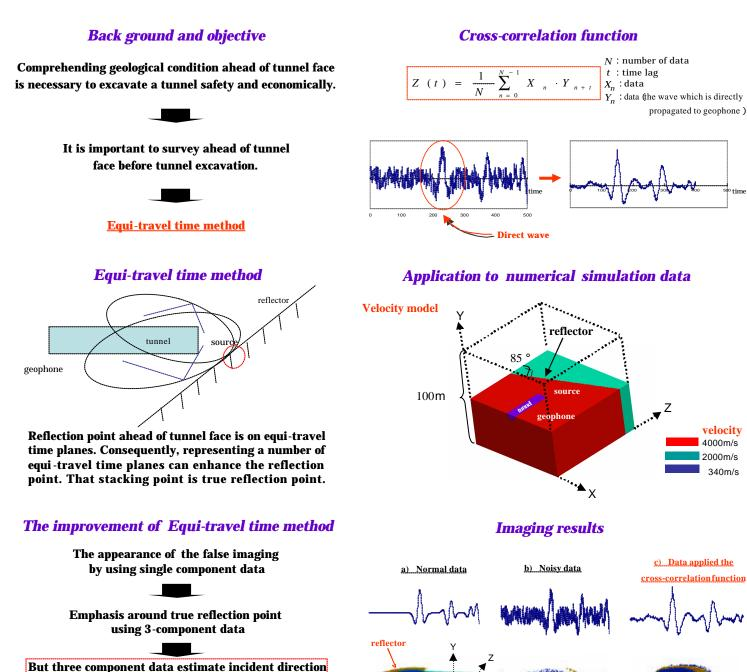
But three component data estimate incident direction of reflected wave from amplitude. So it is difficult to estimate incident direction from noisy data.
